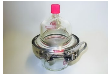
Fig. 2: Migration cell made of glass (one-sided contact)
