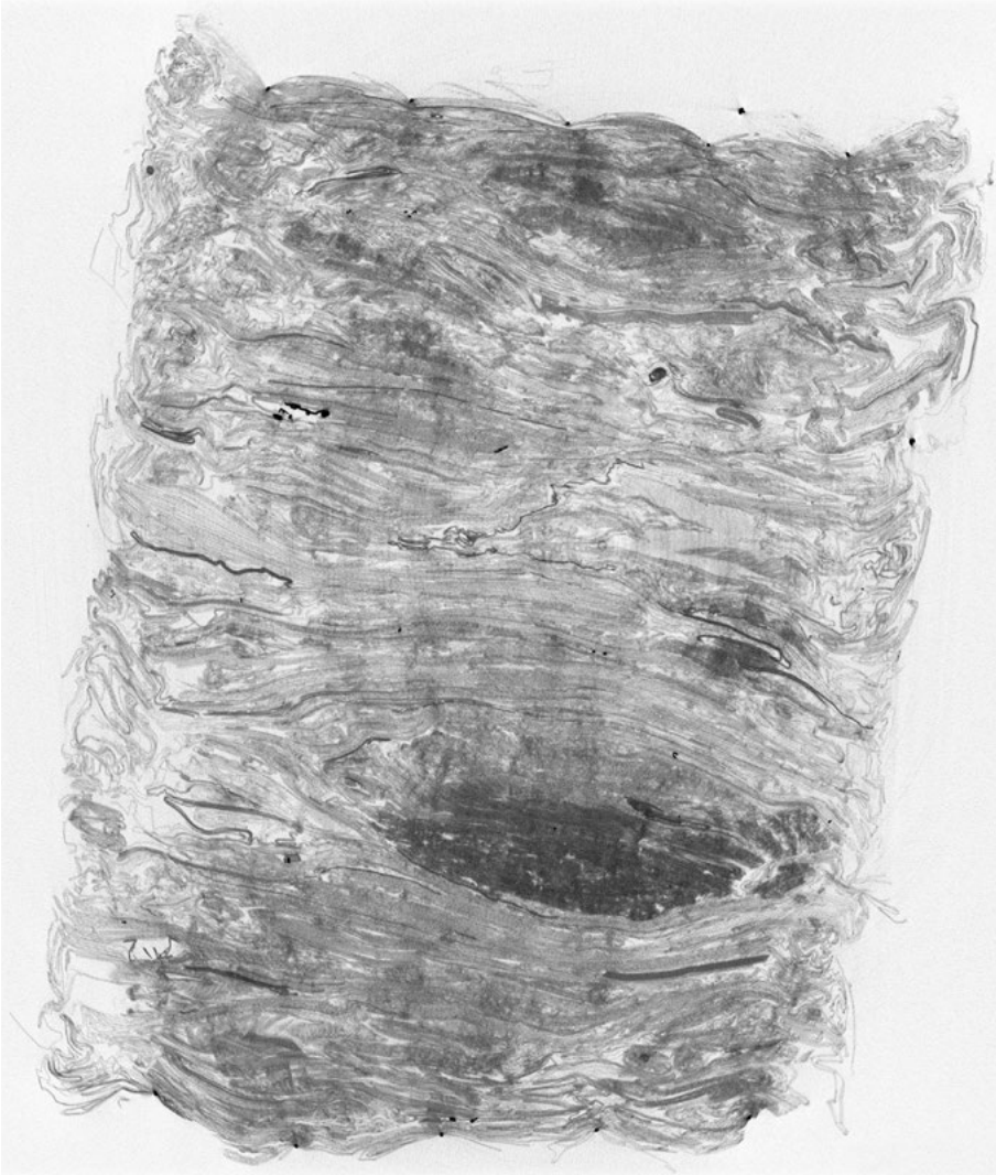
Fig. 1: CT section through a bale of grade 1.04 (darker zones: material with high atomic numbers, black: metals, e.g. wiring)
