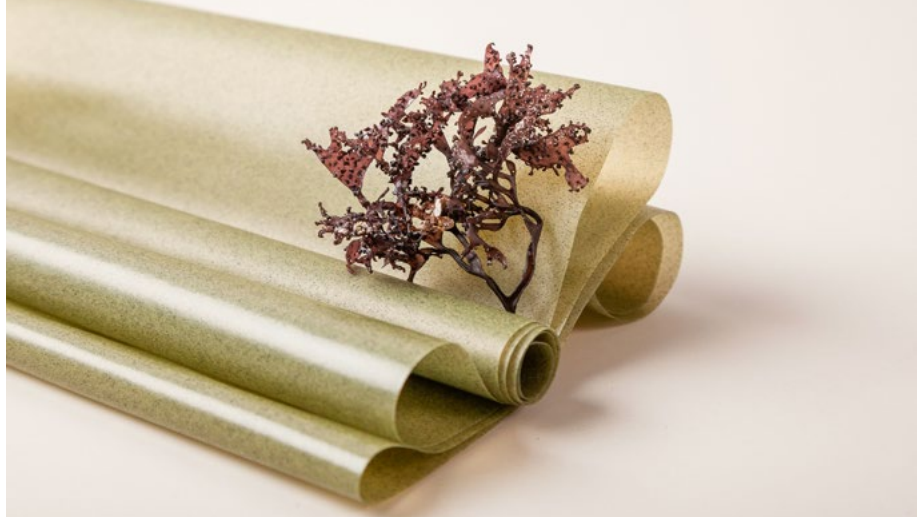
Fig. 3: Alginate film with biological filler additive
